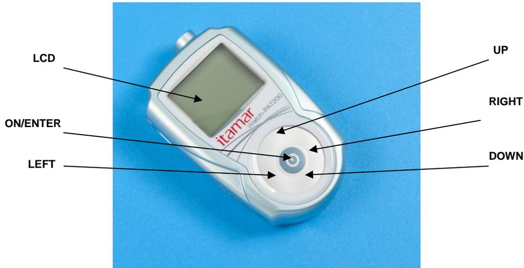
**Figure 3 – The Buttons and Display**
