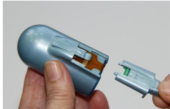
**Figure 8 – Probe Disconnected**
