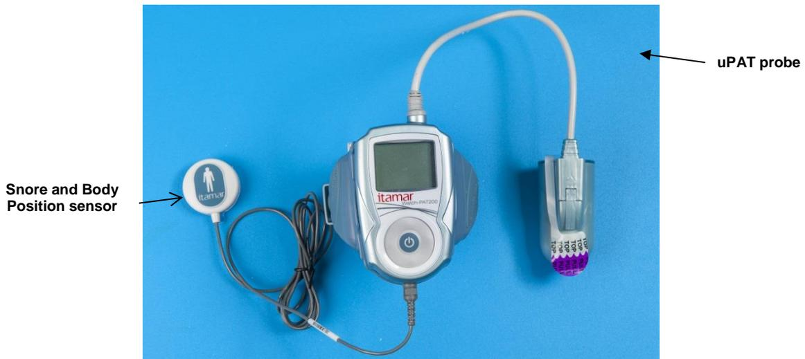
**Figure 9 – WatchPAT™ Fully Prepared**
