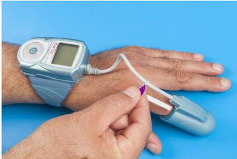
**Figure 24 – Removing TOP Tab**
