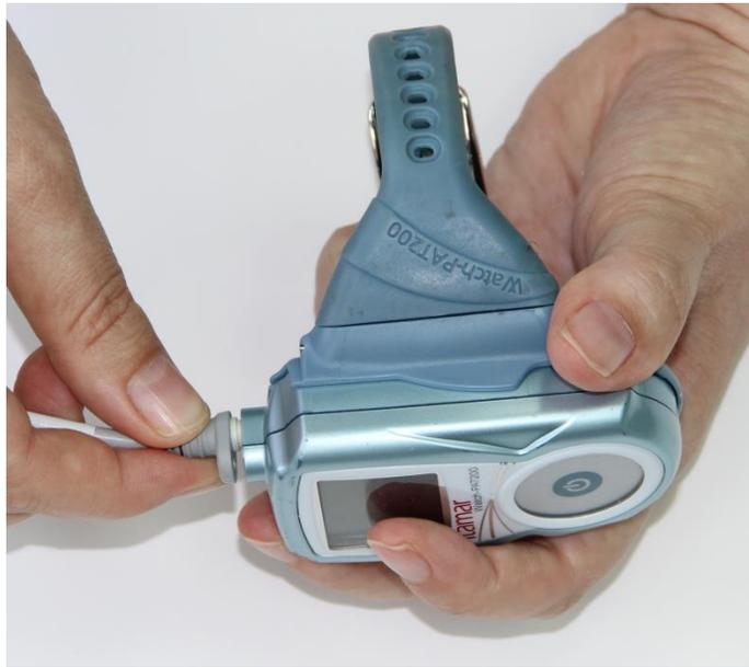
**Figure 18 – Replacing the uPAT Probe**
