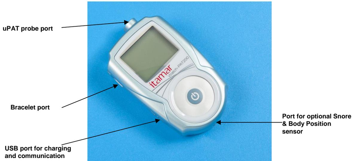
**Figure 4 – Service Ports and Peripherals**
