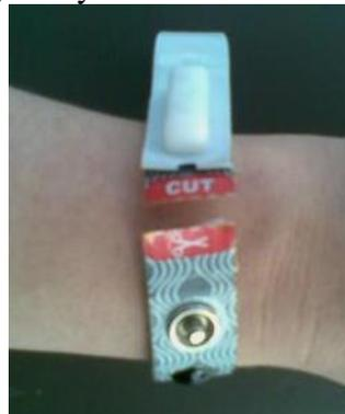
**Figure 15 – Cut the Bracelet on a Specified Location**
