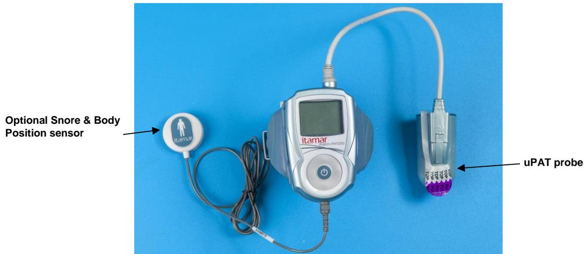
**Figure 2 – WatchPAT™200U Device with Sensors**
